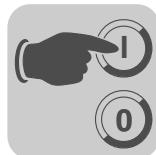
If this parameter is set to the value "ON", the brake can be released even if the drive is not enabled.
