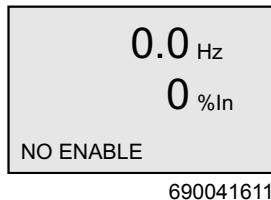
Display for inhibited MOVIMOT® inverter
