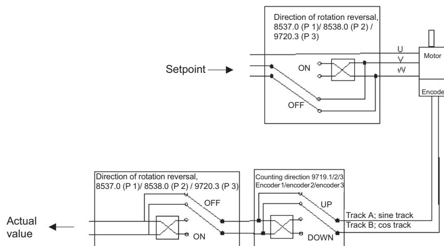
Fig. 44: Behavior of direction of rotation and counting direction
