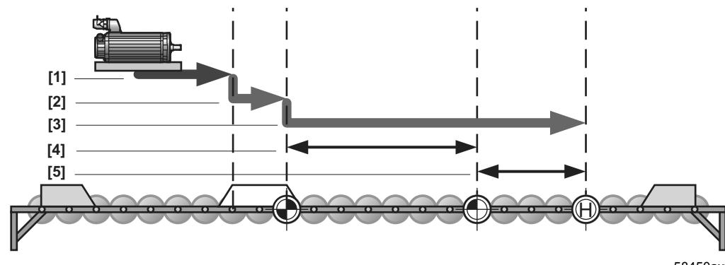
Fig. 30: Reference travel left end reference cam
