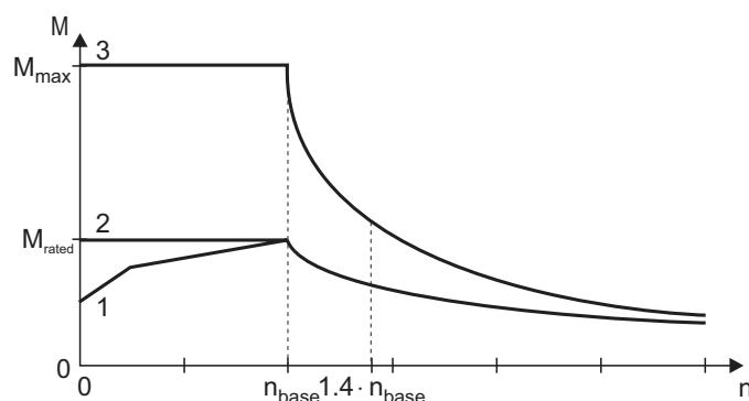
Fig. 9: Sample speed/torque characteristic curve in CFC operating mode
