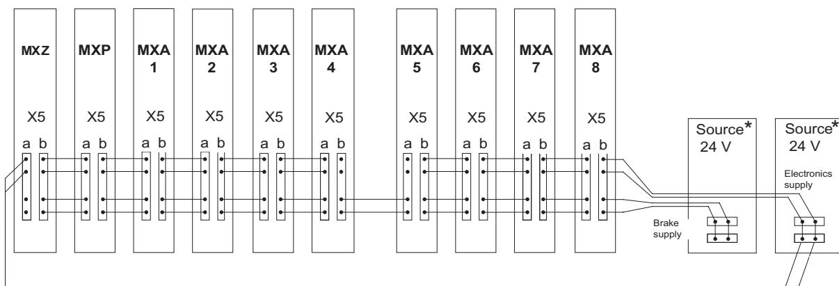
Fig. 15: Example: Two-bus electronics supply
