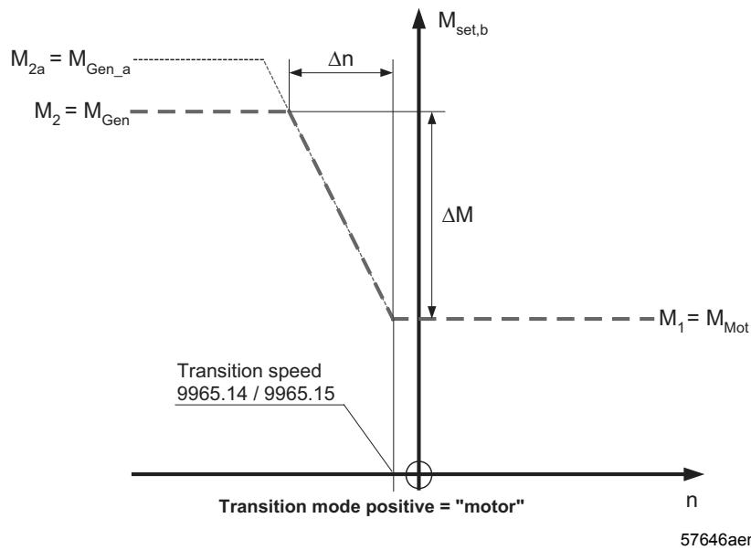
Fig. 50: Positive transition mode – motor
