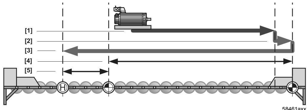
Fig. 38: Reference travel type right fixed stop with hardware limit switch
