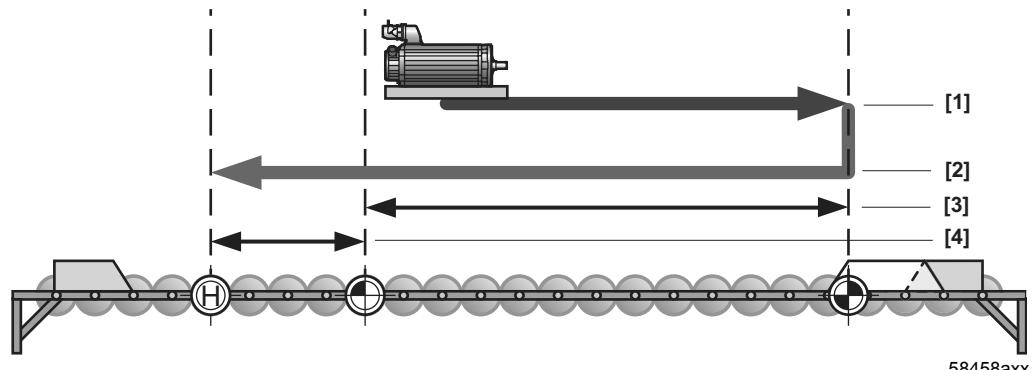
Fig. 35: Reference travel reference cam flush with right limit switch
