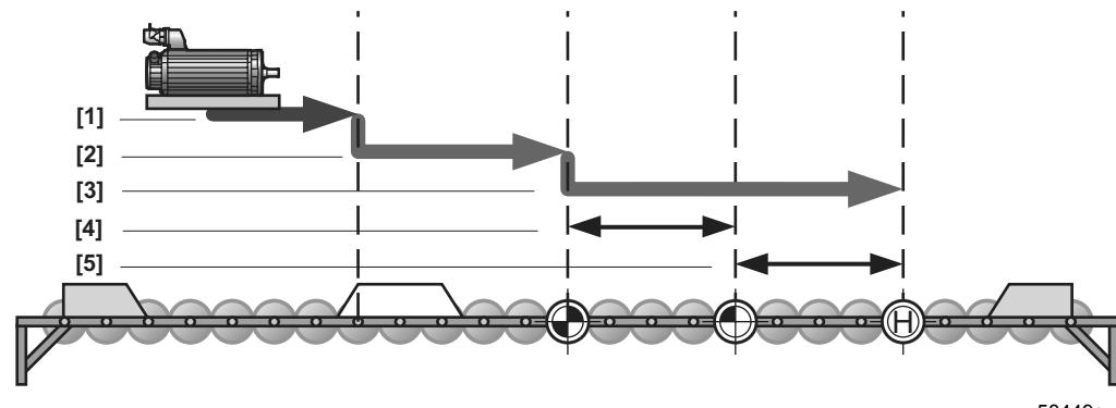
Fig. 29: Reference travel left end reference cam
