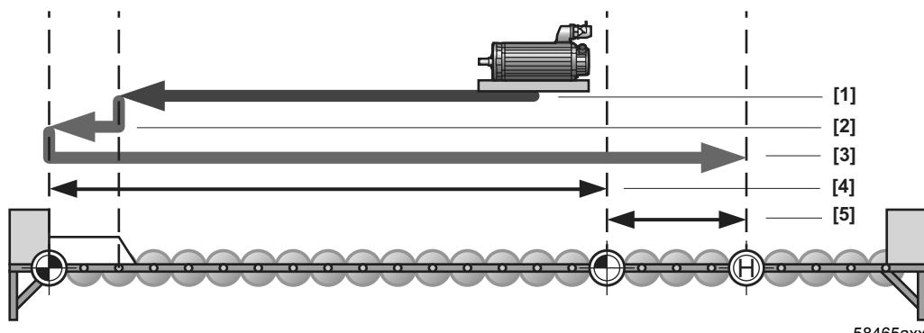
Fig. 42: Reference travel type left fixed stop with reference cam
