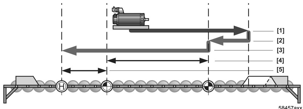
Fig. 34: Reference travel reference cam flush with right limit switch
