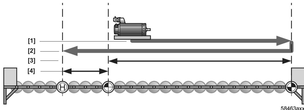
*Fig. 40: Reference travel type right fixed stop*
