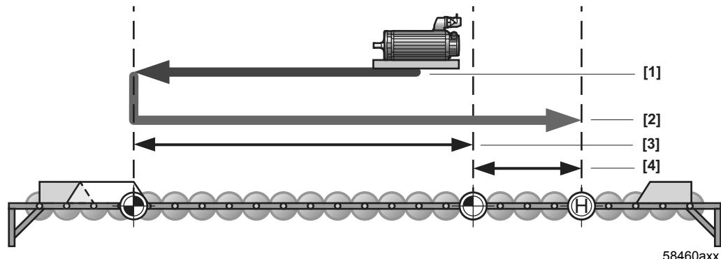
*Fig. 37: Reference travel reference cam flush with left limit switch*
