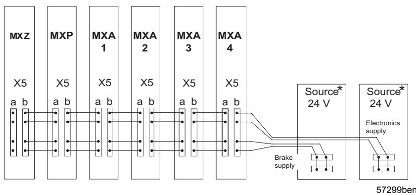
Fig. 14: Example: Single-bus electronics and brake supply
