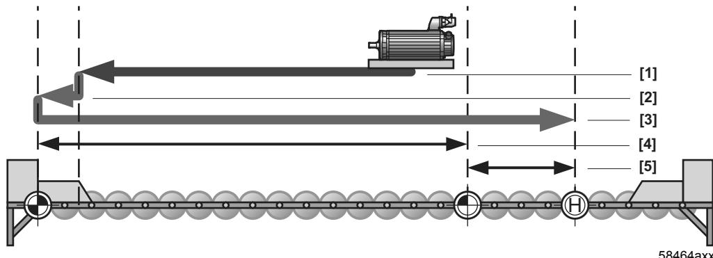
Fig. 41: Reference travel type left fixed stop with hardware limit switch
