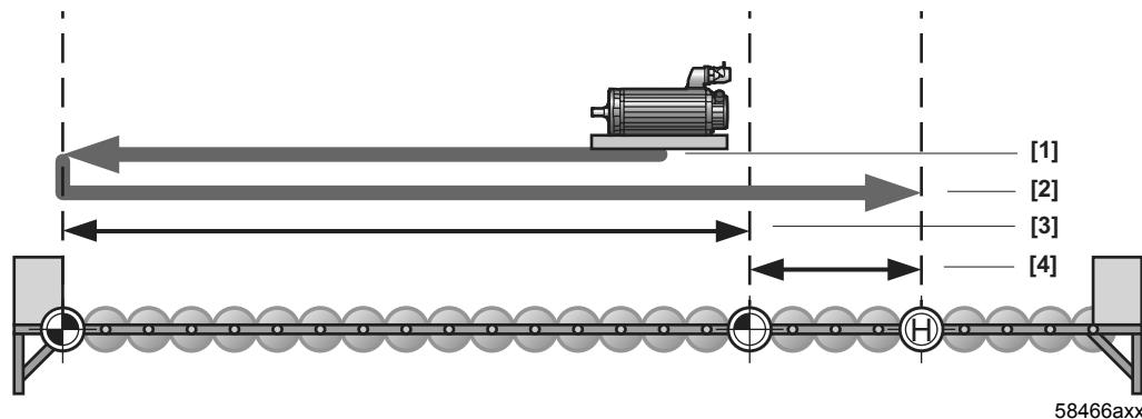
*Fig. 43: Reference travel type left fixed stop*
