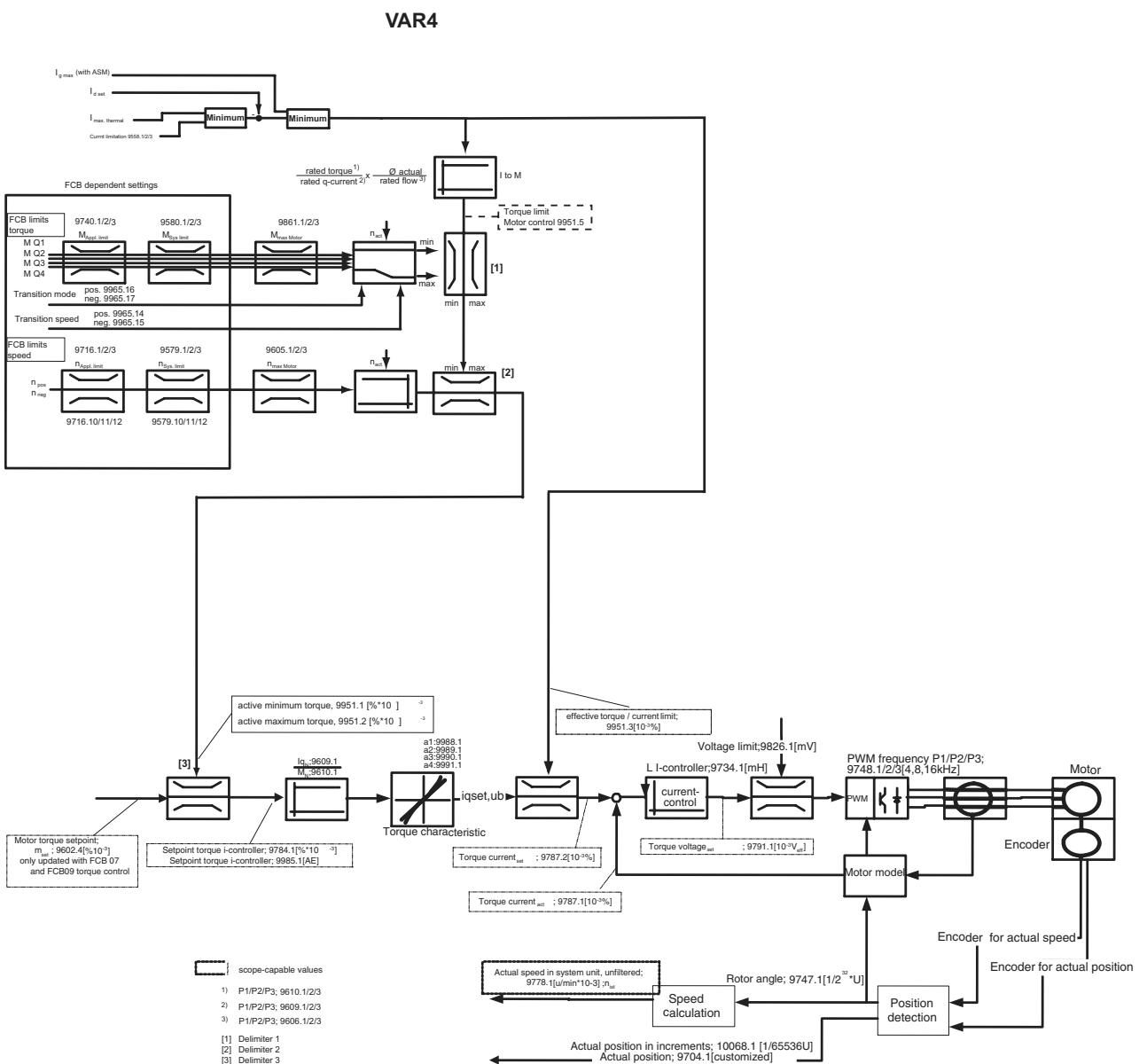
Fig. 21: Torque/current controller
