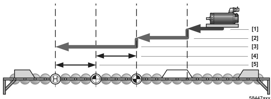
Fig. 27: Reference travel left end reference cam
