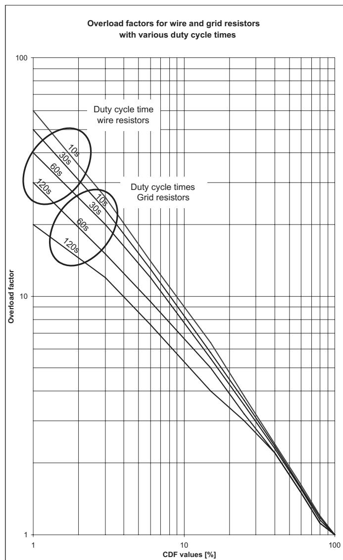
Fig. 10: Overload factors for tubular and grid resistors
