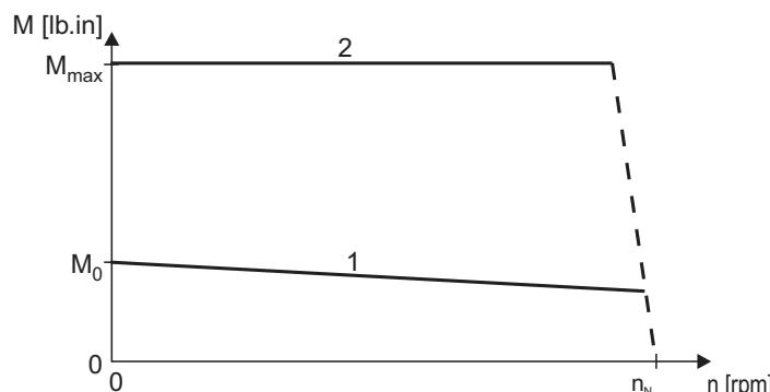
Fig. 8: Sample speed/torque characteristic curve of DS / CM / CMD servomotors
