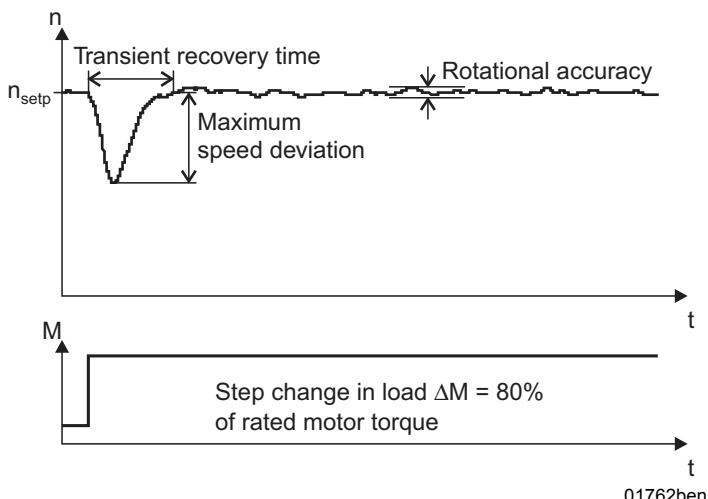
Fig. 7: Features of control characteristics
