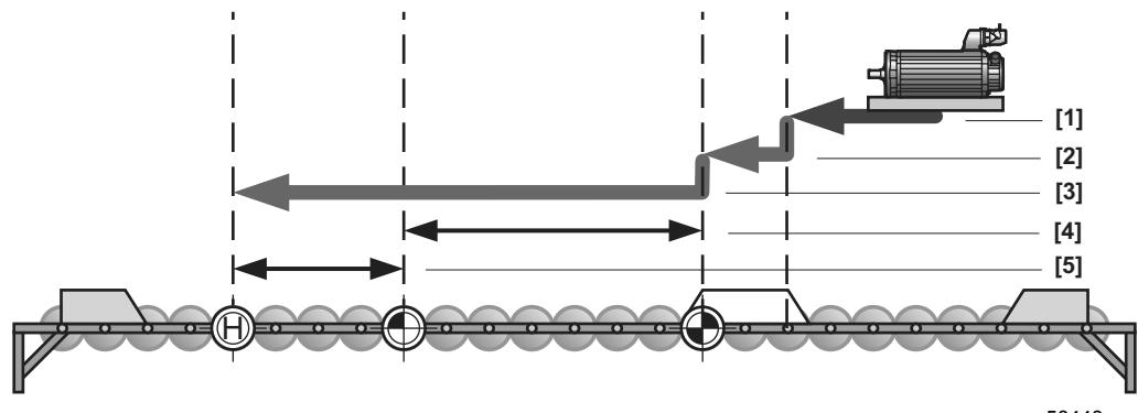
Fig. 28: Reference travel left end reference cam
