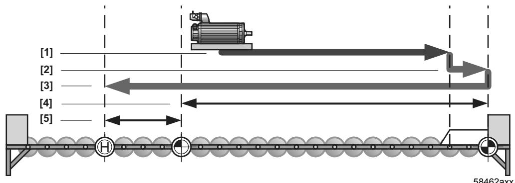
Fig. 39: Reference travel type right fixed stop with reference cam
