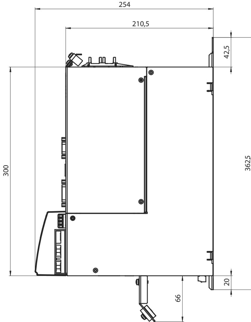
Figure 19: Dimensions axis module BG1, BG2
