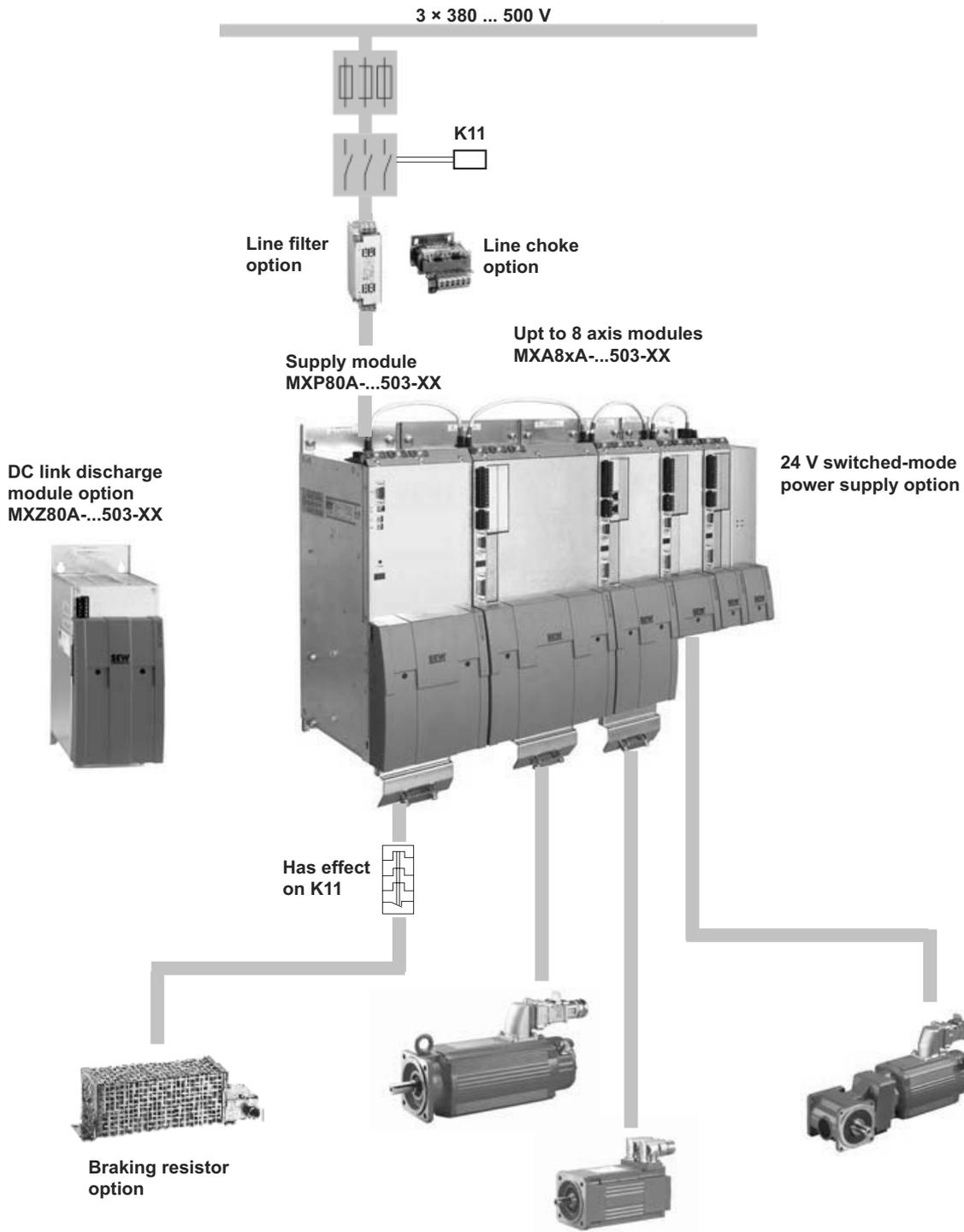
Figure 1: System overview of the power components
