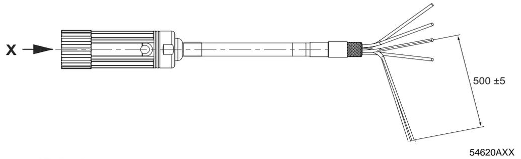
Figure 37: CMP brake motor cable
