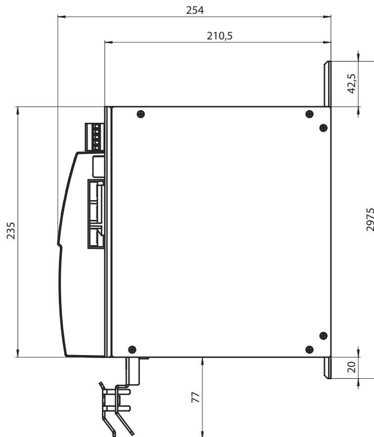
Figure 21: Dimensions DC link discharge module
