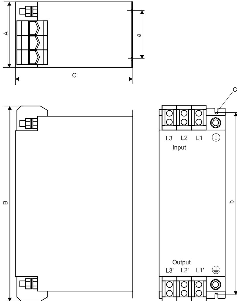
Figure 25: Dimension drawing for NF line filter
