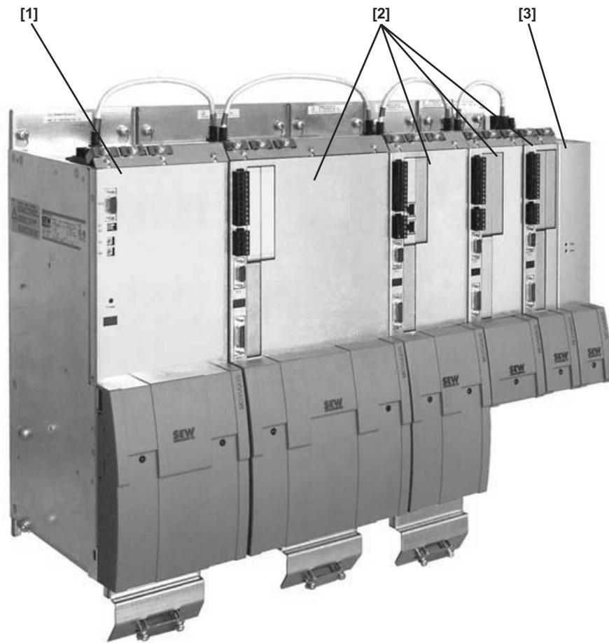
Figure 6: Example of a MOVIAXIS® axis system
