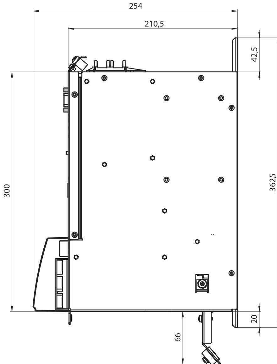
Figure 17: Dimensions supply module BG1
