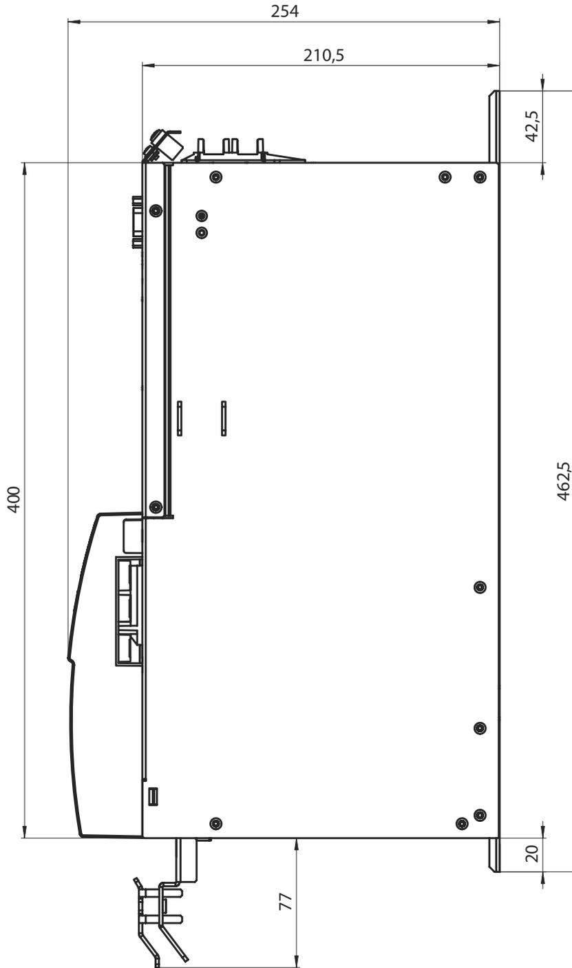
Figure 18: Dimensions supply module BG2, BG3
