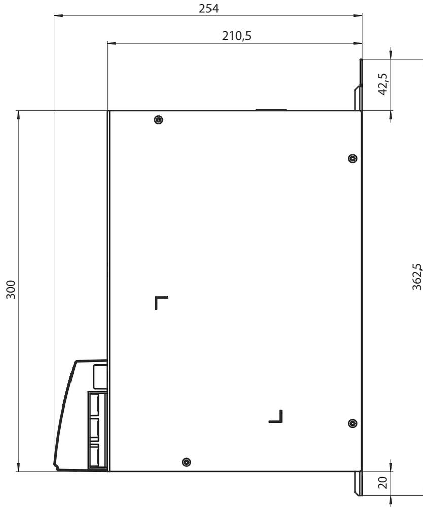
Figure 23: Dimensions 24 V switched-mode power supply module
