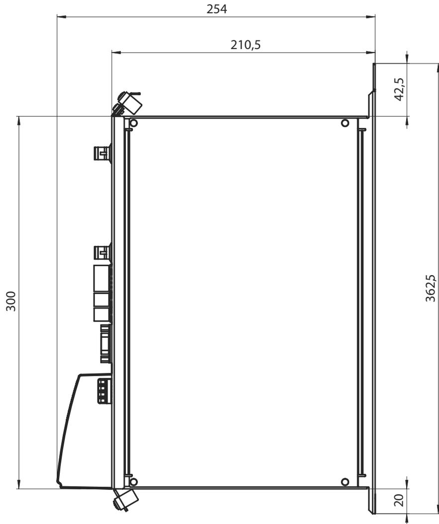
Figure 22: Dimensions master module
