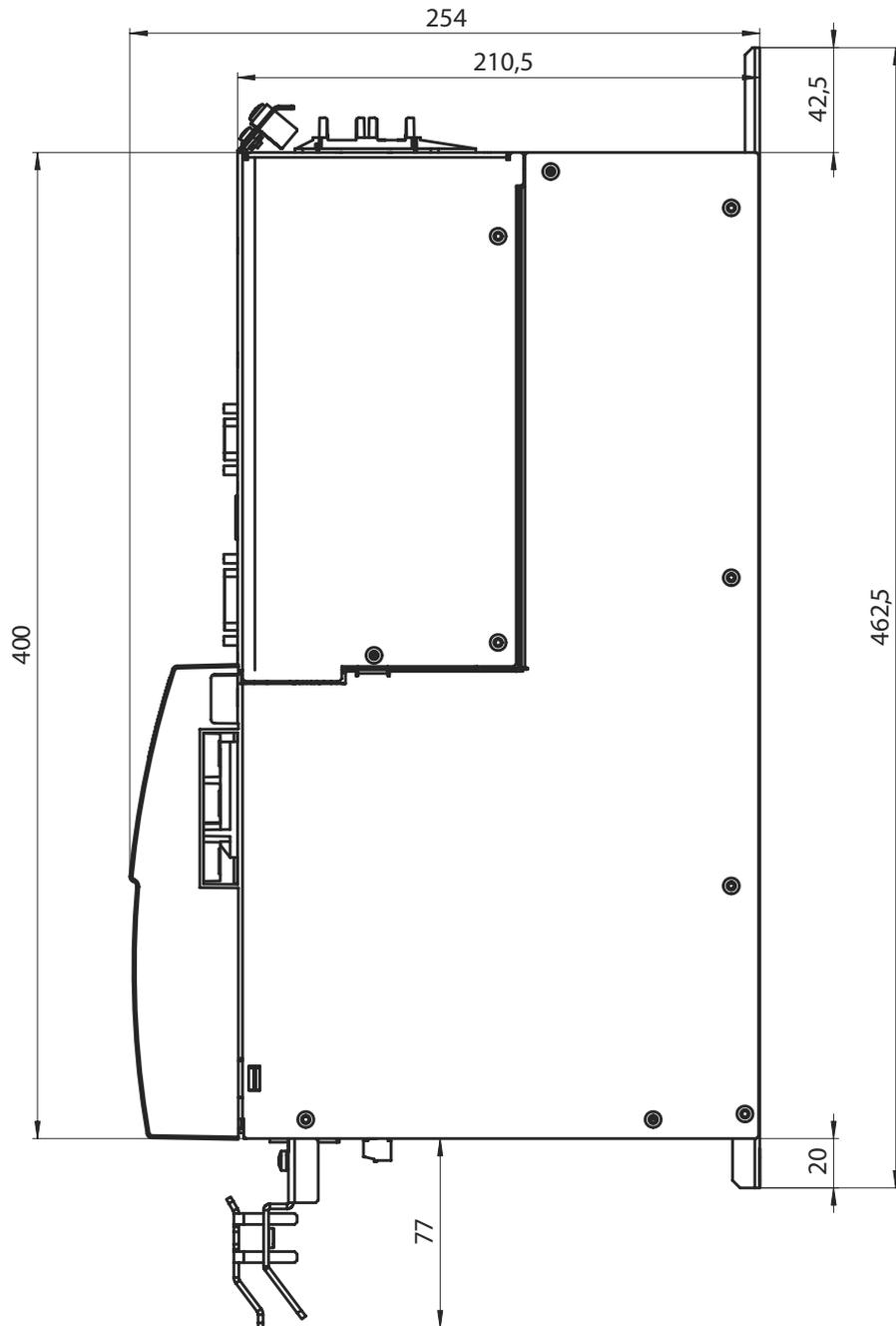
Figure 20: Dimensions axis module BG3, BG4, BG5, BG6
